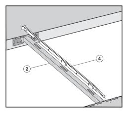
■ Fit the sealing strip ④ into the long slots in the spacer bar ②.
